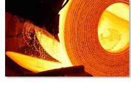
for the manufacturing of steel components, various metal products, and as feedstock for cold-rolled steel production. The high demand and diverse applications dictate certain variations in the chemical composition and physical-mechanical properties of hot-rolled steel coils. At Zaporizhstal, hot-rolled coils differ in steel grade, chemical composition, mechanical properties, geometric dimensions, and the final product's weight.
